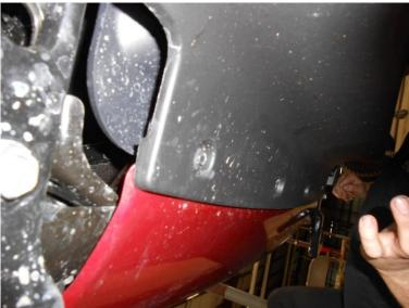
2. From the bottom of the vehicle, unscrew the fasteners holding the OEM tow hooks to the frame. It is a good idea to support the OEM bumper during this process
