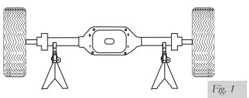
2. Lower the axle or raise the body of the vehicle until the springs are completely extended (wheels hanging).
