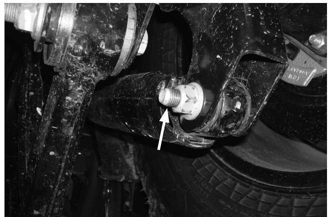
Mark spring location in reference to upper and lower spring seat. Sample of passenger's (right) side shown.
