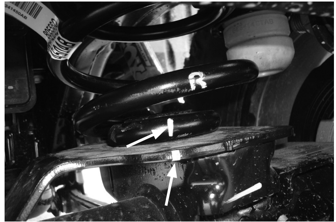
Mark spring location in reference to upper and lower spring seat. Sample of passenger's (right) side shown.
