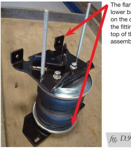
The flanges on the lower bracket must be on the opposite side of the fitting that is on the top of the air spring assemblies.
