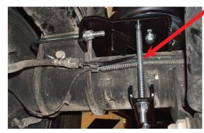
Check driver's (left) and passenger's (right) sides to make sure the hard brake line is not rubbing on the carriage bolts. Adjust by pushing on the line to gain clearance if necessary.
