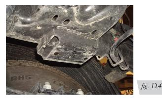
Install the upper frame brackets (B) onto both sides of the frame with the M10-1.5 x 35 button head cap screws (J) making sure the cutout in the brackets face inboard, away from the tire (Fig. D.5). Torque the hardware to 37 lb.-ft. (50Nm).
