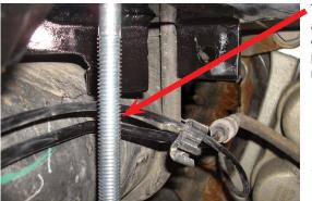
The carriage bolt is always on the outside of the brake line on the passenger's (right) side, regardless of the year.
