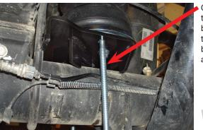
Carriage bolt must be on the outside of the hard brake line and axle for this model that has the brake line flush to the axle.
