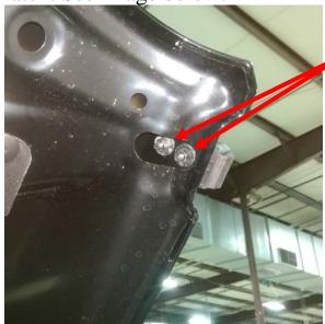
Remove using 10mm socket.
