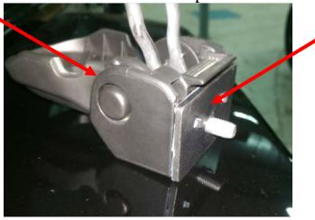
**6.** Reinstall hood latch with spacer.
