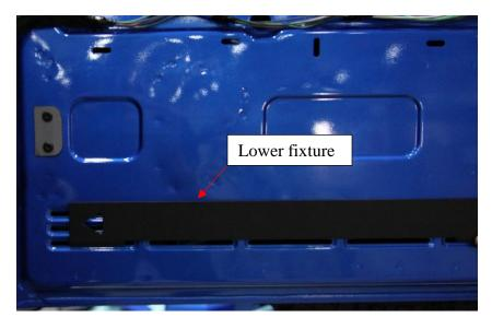
5. Next place rear door plate in place, lining the door plate up with installation fixtures as shown below.
