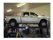
1) Raise the vehicle up on a hoist or rack to working height. If you do not have access to a hoist or rack, raise the vehicle and support securely with jack stands.
