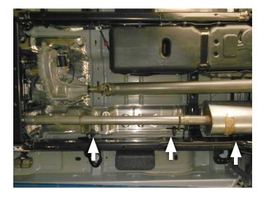
5. If your vehicle has electrical wiring routed along inside face of right frame; carefully release harness from frame by unclipping it. Then use cable ties to secure it to top of frame (or to harness already on top of frame, as shown).
