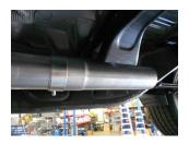
2) If installing the system on a Crew Cab truck with a 6.5' bed, place extension pipe **#TB700S** onto the back of the **#26429S** inlet pipe, place a provided clamp onto the slip-fit and tighten enough to hold in position. This extension pipe will not be used on Double Cab or Crew Cab-5.5' bed models.
