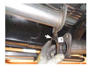
Secure each flange using bolt (3) through flat washer
