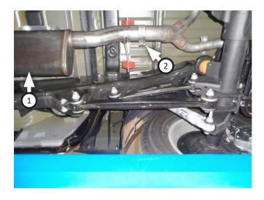
8. Place gasket (removed step 5) between muffler and factory pipe then hang muffler wire hanger into rubber isolator. Connect grounding wire to muffler.
