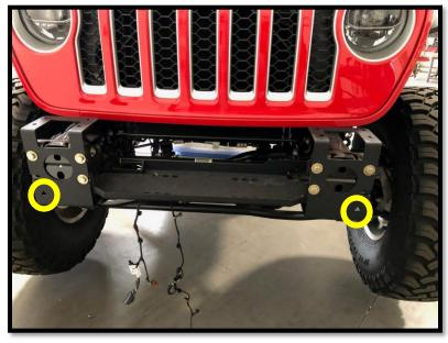
4. Prior to placing bumper on brackets, install fog light adapters and fog lights at this time. This bumper only accepts fog lights with the 4 mounting holes.
