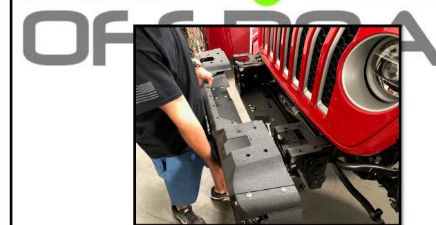
6. Install light covers over fog light holes using supplied bolts.
