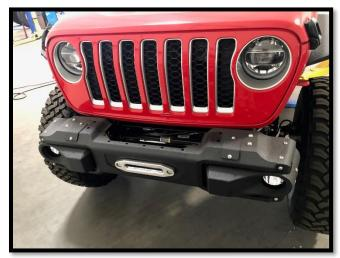
7. Install bull bar and winch plate cover if no winch used.
