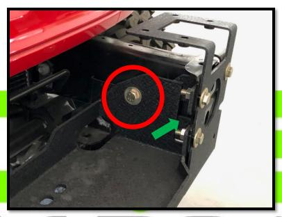
3. Place bumper mounting brackets over frame rails noting orientation of the triangles on each side. NOTE: If you are using the factory Jeep tow hooks, place them on the back side of the frame plate with the studs facing away from the Jeep (green arrow in image on step 2. Use Studs with nuts to secure brackets to frame)
