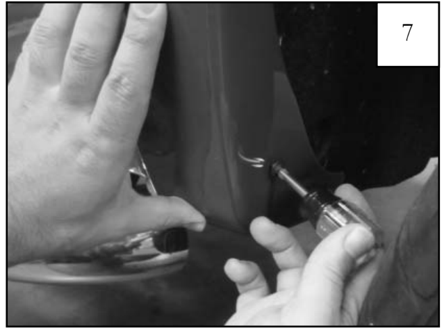
Place flare on vehicle and start supplied Screw (SW1-0056) through two bottom rear holes in flare and into factory hole in front of wheel well. Do not tighten.
