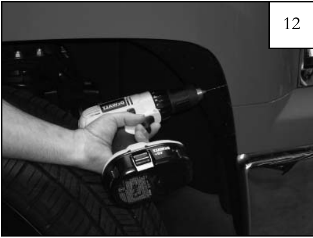
Using a 3/32" drill bit, drill pilot holes at the marks made in Step 11.
