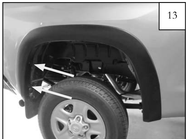
Start two supplied 20mm Hex Screws through the rearward most holes of flare and into the factory hole in fender.
