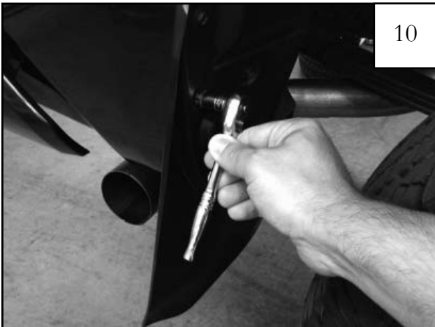
Using a socket wrench with a 10mm socket, factory screw second from the top of the mud guard.
