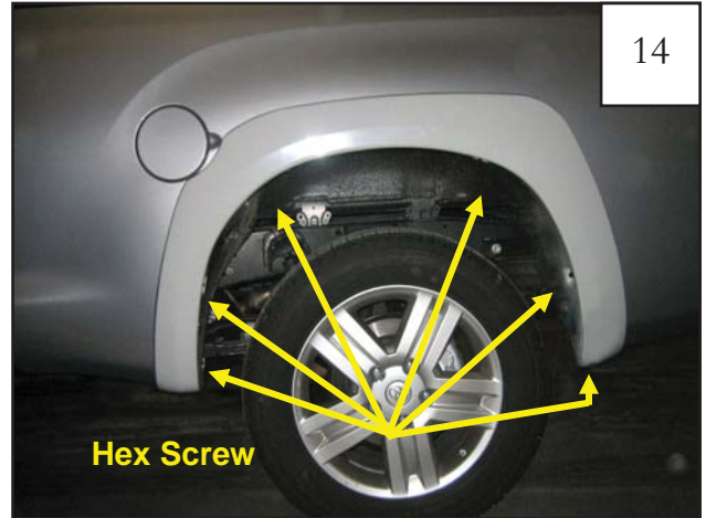
Hold the flare firmly on the fender. Start a supplied Hex Screw through each hole in flare and into hole in fender (six places).
