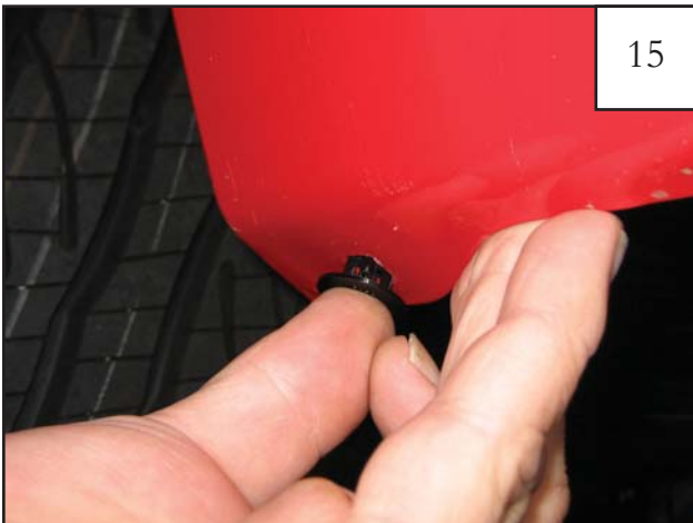
Note: If the lower rear wheel well does not contain a plastic grommet, insert a supplied one into the factory hole as shown.
