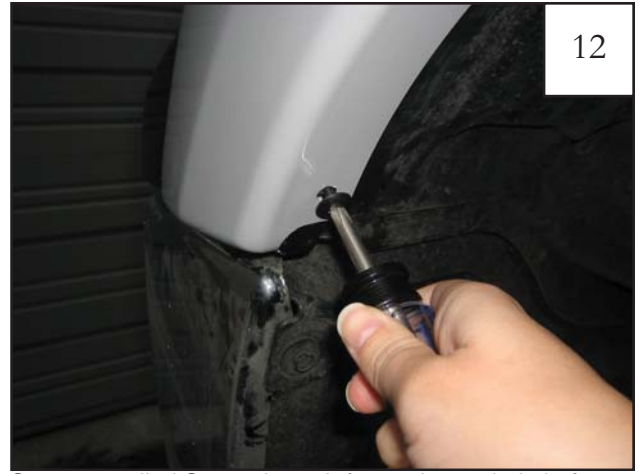
Start a supplied Screw through forward-most hole in flare and into "U" Clip installed in Step 8. Note: For the Limited version, install this screw directly into hole in fender. Ensure flare is properly positioned and tighten all screws.
