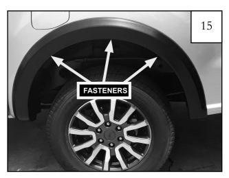
Hold flare to vehicle and install (3) 1/4" panel retainers (RV1-P008) into the wheel well holes indicated. Press firmly on the flare while installing fasteners.
