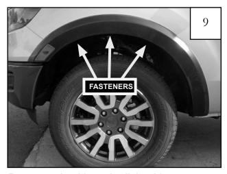
Reconnect the side marker light wiring connector and set the flare in place. Hold flare to vehicle and install (3) 1/4" panel retainers (RV1-P008) into the wheel well holes indicated. Press firmly on the flare while installing fasteners.
