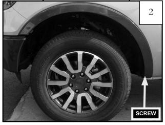
Remove (1) factory installed screw from the rear of the fender trim using a T-25 Torx driver. The screw will be re-used to install the front flare.
