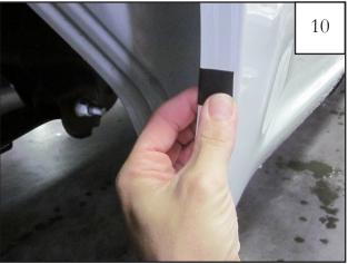
Wrap a Foam Tab (MT1-0034) around the wheel well sheet metal, centered over each of the upper four marks made in Step 9. Place a Mylar Tab (MT1-0014) at the mark made on the lower front of the wheel well.
