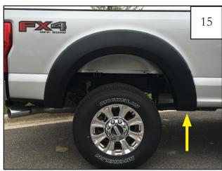
Start a supplied screw (SW1-0050) through the flare into the clip installed in Step13. Tighten all screws.
