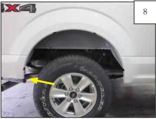
Remove factory fastener from rear of wheel well. Thoroughly clean the vehicle sheet metal and inner flange prior to installation.
