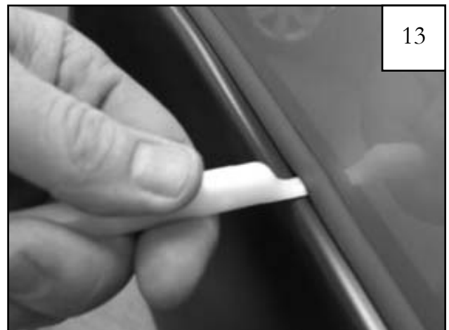
13 Using flat end of supplied Edge Trim Tool (ET1-0002), seat edge trim against flare by inserting straight end between edge trim and flare at one end. Next, slide around entire edge to the other end.
