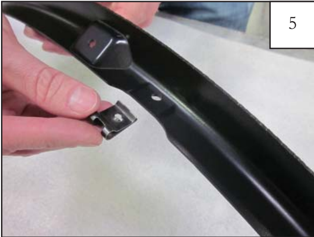
Attach 3 "U"clips (CL1-0022) to the inner bracket as shown.
