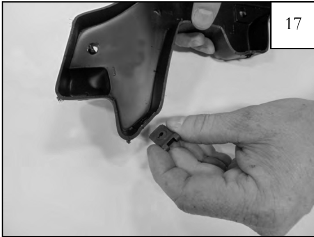
Install a U-clip at each clip location on the inner pieces, centering them on the predrilled holes with threaded portion on inside (9 locations). NOTE: Clips may slide out of place. Try pinching the metal tightly onto the inner piece with pliers.
