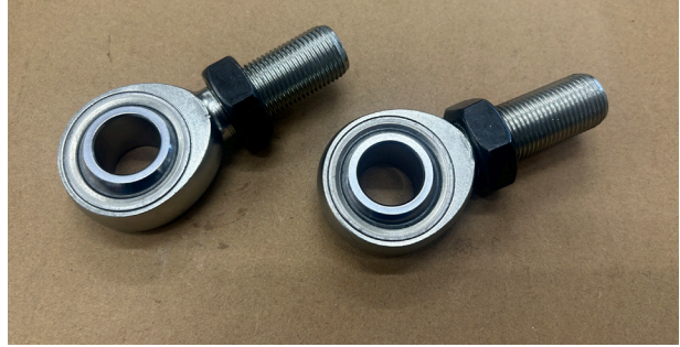
Fig. 10: Install the 3/4" jam nuts.
