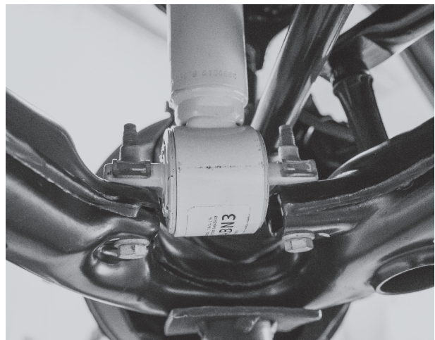
Fig. 6: Remove 2 bar pin bolts.
