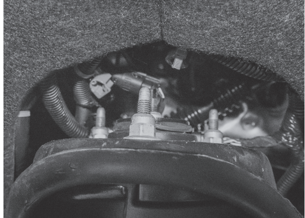
Fig. 2: Loosen the 3 upper mount nuts.
