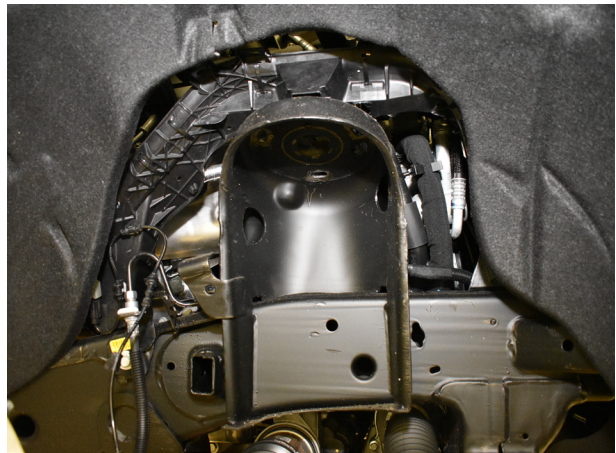
Fig. 8: Remove ABS wire then remove UCA.
