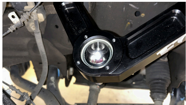
Fig. 16: Assemble uniball joint.
