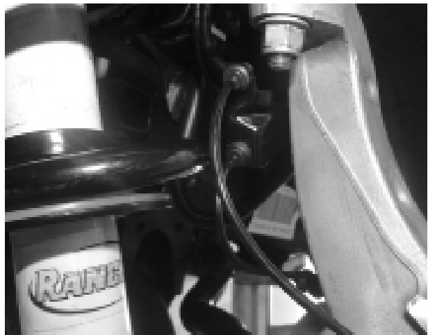
Fig. 4: Unclip ABS wire.
