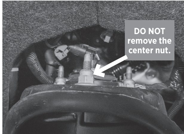
Fig. 7: Remove the three nuts, NO NOT REMOVE CENTER NUT.
