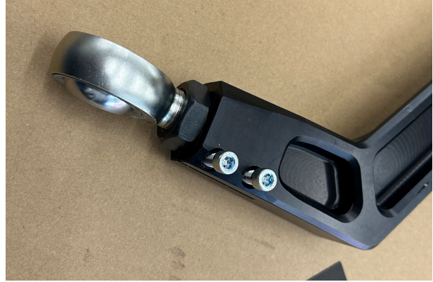
Fig. 13: Loctite and install pinch bolts.
