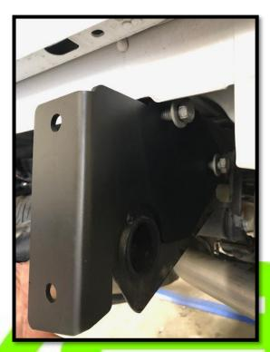
5. Using provided hardware, mount the bumper to the brackets and leave loose.
