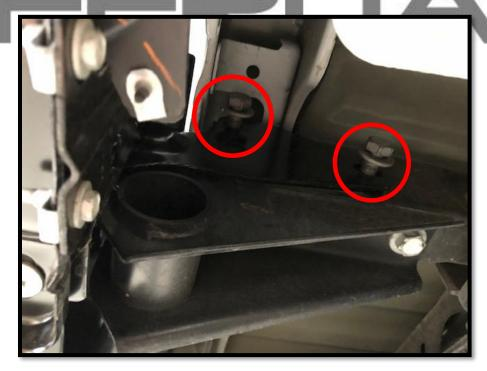
4. Once bumper is removed, install the new bumper brackets onto the frame of the truck using factory hardware. NOTE: Leave all hardware loose until the end. This will allow for adjustment later on.
