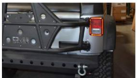
Step 13: Install tire stud and license plate holder with the six 12 mm bolts provided.
