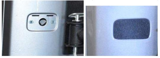
Step 15: Remove driver side brake light housing and disconnect wires, set aside you will be reinstalling later.
