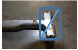
Step 7: Take the new upper body hinge with the elongated bolt hole and take a round file and remove powder coating from holes so the new hinge pins and bolts will fit through. You may also need to file the powder coating away from the inside of hinge so that the rear door hinge will fit inside.
