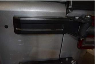
Step 1: Remove plastic hinge covers from rear door hinges.
