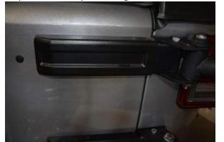
Step 11: Reinstall plastic hinge covers on rear door.
