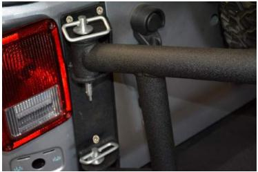
Step 20: Remove the quick release pins and pull the tire carrier to the open position. The body mounting bracket should be securely mounted to the body. Mark the last two mounting holes that were covered by the tire carrier when closed. Use center punch and hammer and lightly punch the center of your mark, drill pilot holes with 1/8" drill bit and then drill to final size with 5/16" drill bit.
