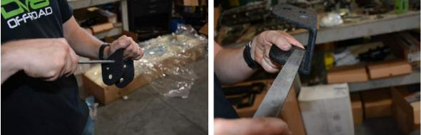
Step 8: Take the door hinge and body hinge and slide them together so that the hinge pin holes line up and slide new hinge pin through and secure with nut.
