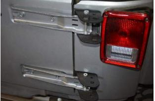
Step 10: Install the hinge to the door with the two 13 mm bolts. Install the hinge stopper bolt through the upper hinge, this bolt keeps the tire carrier from opening too far.
