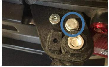
Repeat the process for the lower door hinge. (note: Lower body hinge bracket does not have an elongated hole.)
