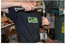
Step 6: Pull the hinge apart and discard the portion of the hinge that previously bolted to the body.
