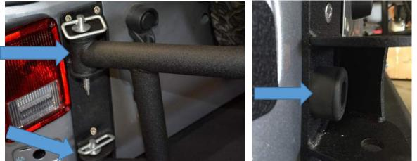
Step 21: Install the rubber bumper stops to the last two mounting holes with the provided hardware using the two button head bolts and secure with nuts. (note: Do not over tighten or you will collapse the stopper.) The rear body mounting plate is now fully installed. Reinstall brake light housing and don't forget to plug the rear light harness back into the housing.
