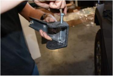
Step 9: Install the new hinge to the body with the 3 torx head bolts first.
