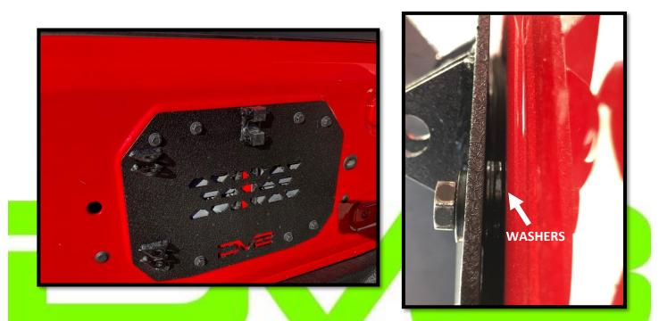
9. Install the carrier stopper onto the carrier as shown using provided hardware.
