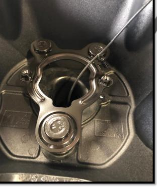
16. Using a punch, lightly tap out the factory camera mount. NOTE: This is plastic and so be careful and punch out the two holes in the center equally.
