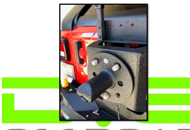
19.Place spare on carrier. Open and close carrier to sure all parts are moving properly.
