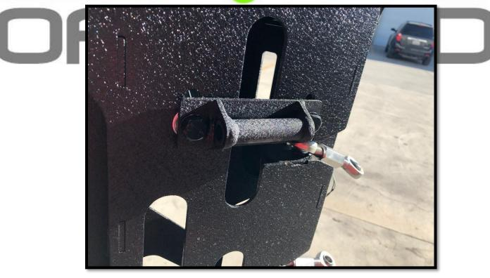
10. Install heims onto carrier door. With the door closed and parallel with the rear hatch plate, adjust heims so that they line up with tabs on rear hatch plate.
