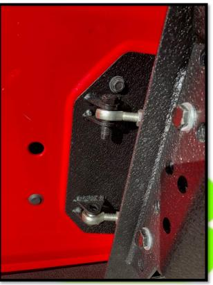
11. Once installed, if there is any play on the carrier when the hatch is closed, either the heims need to be adjusted inwards, or you can space the stopper on the carrier arm with one or two washers so there is a firm fitment when closed.
