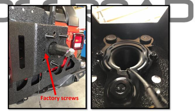
18. Using the provided camera enclosure, cover the camera and bolt using supplied flush mount allen head bolts.
