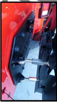
**12.** Remove factory third brake light from stock carrier. Attach to new carrier using (4) factory screws.
