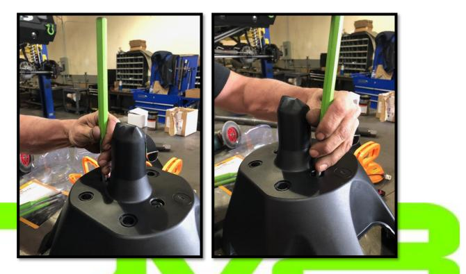
**17.** If using a camera, place the factory camera mount (plastic) though the holes. Place the factory stud plate behind it. Secure using factory bolts.
