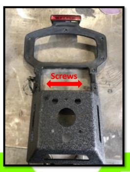
13. If you are running a rear camera you will utilize the factory camera bracket (plastic) and the provided camera enclosure. If you do not have a camera, you will utilize the block off plate.
