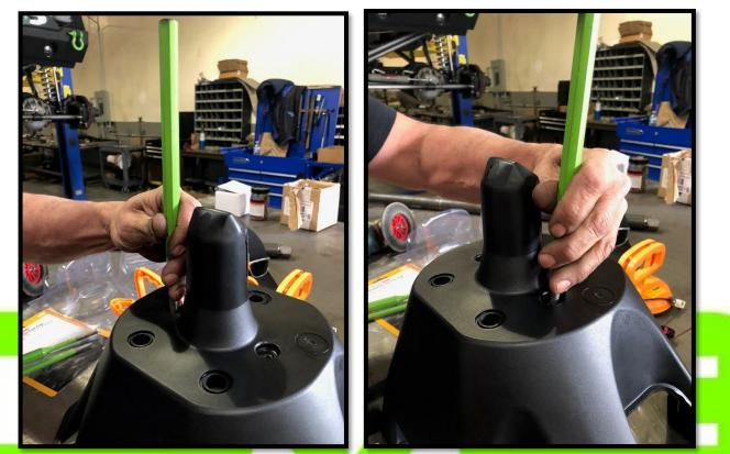
14. If using a camera, place factory camera mount and camera (plastic) though holes. Place factory stud plate behind it. Secure using factory screws.
