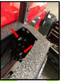
18. Tighten down (4) four tire mount bolts. Ensure all hardware is secure. Install plastic bumps on side of carrier. Plug in camera and third bracket light. Attach tire and test door.
