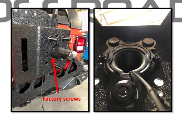
15. Using the provided camera enclosure, cover the camera and bolt using supplied flush mount allen head bolts.
