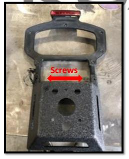
11. If you are running a rear camera you will utilize the factory camera bracket (plastic) and the provided camera enclosure. If you do not have a camera, you will utilize the block off plate.
