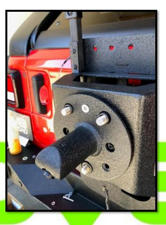
16. Place entire assembly on spare tire and attach using stock lug nuts. Take entire assembly and tire, and hold it up to carrier. Since there is many holes for adjustment, find what ones best fit your tire size.
