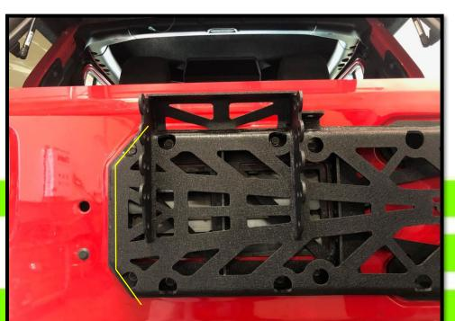
10. Remove the factory third brake light from original tire carrier by removing the (4) screws.a. Replace this onto new DV8 tire carrier.
