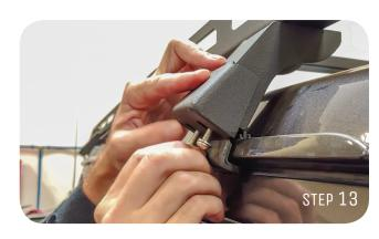
STEP 14: Making sure the rack is centered on the top, tighten up the front and back gutter clamps on each side first. This ensures the 2 other clamps move as needed to fit properly. Then tighten the 2 middle clamps.
