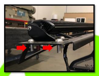
3. Once loosely attached, bolt the other side of the rack as well. With additional help, lift rack onto bed of Gladiator. Align the two holes on front of the truck. If you haven't already, remove factory bolt from this position since you will reuse it for the rack.
