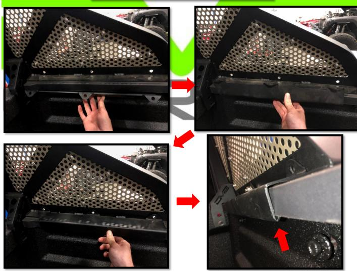
6. Tighten down the front bed bolt, then tighten down the clamps until rack is secured. The hole above the factory bolt can either be thru bolted or can be used to add an eyelet for a tie down point.
