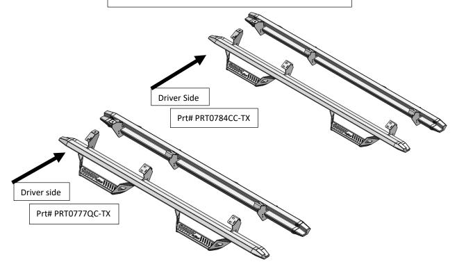
**Step 2** Beginning with the driver side, carefully raise the step rail up and match the brackets with the factory mounting locations. Next, starting with the center bracket and using the supplied M8x25mm hex bolts, 5/16" flat washer and lock washer start and leave loose.
