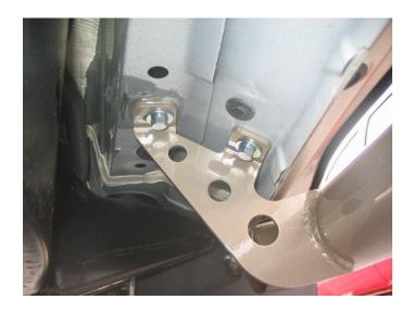
**<u>Step 4</u>** After finial adjustment, torque each bolt to 17 ft/lb – 20 ft/lb.
