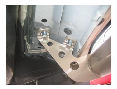
**Step 4** After finial adjustment, torque each bolt to 17 ft/lb – 20 ft/lb.
