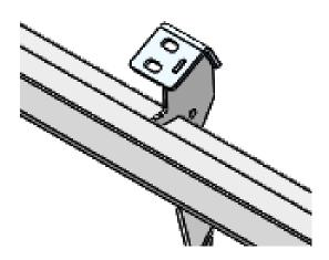
**Step 5** Start all remaining M8x30mm hex bolts in each bracket and leave loose.
