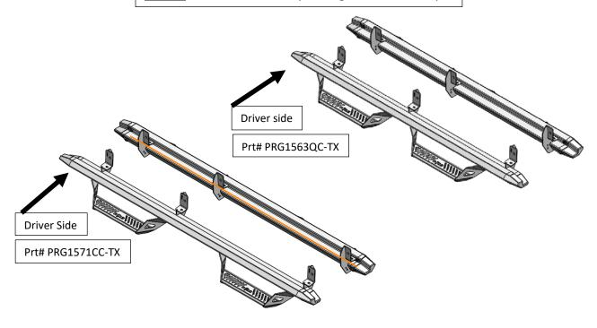
**Step 2:** Starting with the driver side, locate the rubber body plugs on the underside of the body. There will be four sections of two plugs each. One near the top of the body and one near the bottom. (. **NOTE**: Some applications use three brackets per side and some use four brackets per side.) **Fig. A**
