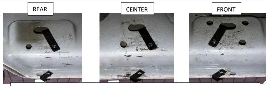
U-clip positioning. NOTE: Clip orientation will be the same for passenger side.
