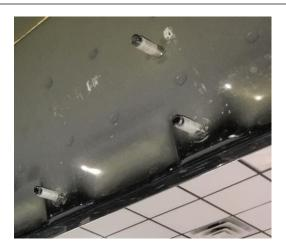
**Step 4:** Carefully install the Predator Pro step to the three factory attachment points using the provided M8 flanged hex nuts. Leave finger tight for now.
