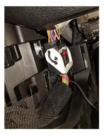
**3.** Disconnect the door power window and lock wiring harness if applicable.
