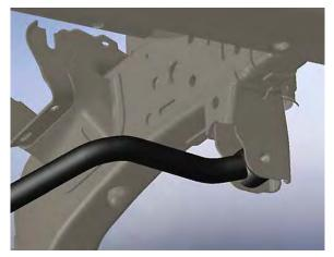
O Loosely install the original mounting hardware.
