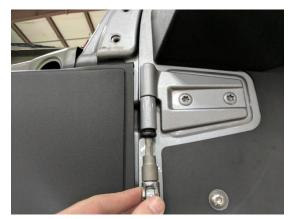
**2.** Remove the door restraining strap webbing by separating the nylon loop from the metal hook.
