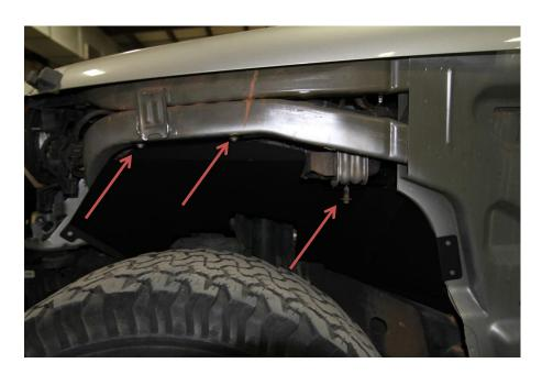
**3.** Mark the three lower mounting points in preparation for drilling the piolet holes.
