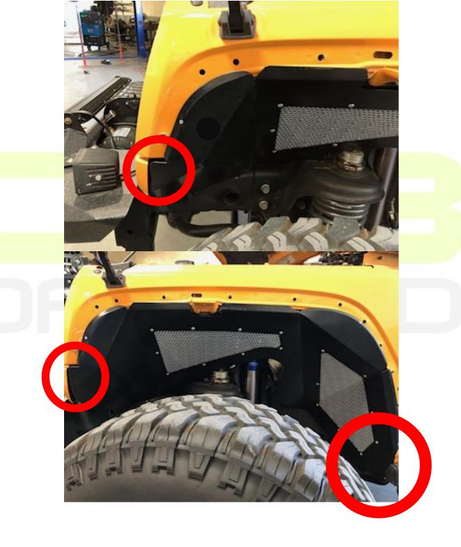
**6.** Once aligned, mark holes in inner fender on Jeep body. Using 1/8" drill bit, drill marked holes in body. The inner fender will sit on top of the edge of the wheel well.
