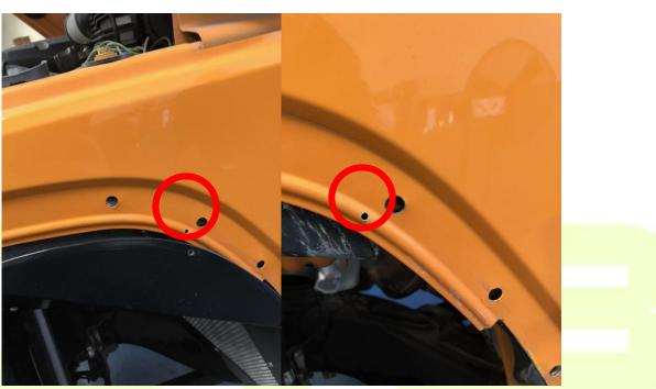
**7.** Realign inner fender. Using rivet gun and provided rivets, install the inner fender. Ensure proper inner fender alignment prior to install rivets.
