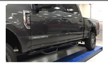
**Step 1:** Starting with the Driver Side. Remove all 8mm flange nuts from the 8mm factory threaded studs to remove the OE running boards. Repeat for passenger side. **(Fig.A).**
