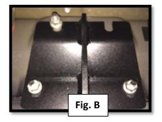
**Step 5:** Staring with the rear bracket, push up towards the pinch weld so the 3" main bar is as high and tight to the body as possible. Tighten all three 8mm flanged nuts.
