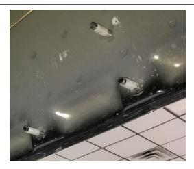
**<u>Step 4</u>**: An additional person is recommended for this step. Carefully install the Hoop step to the three factory attachment points using the provided M8 flanged hex nuts. Leave finger tight for now.
