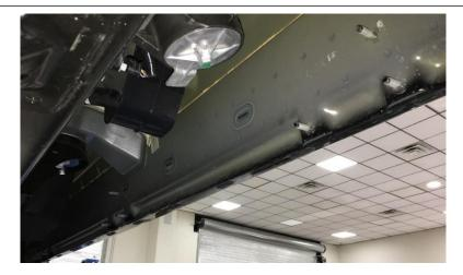
**<u>Step 3</u>**: On the inside rocker panel there will be three-attachment point consisting of three 8mm studs coming out from the panel. These studs may be covered in paint and will need to be cleaned before the installation.
