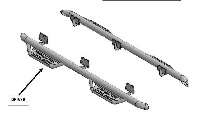
Step 2: Starting with the driver side, remove any steps and old hardware from the vehicle.
