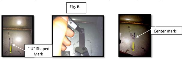
**Step 9:** Remove clip. Use a ½" drill bit and drill out the center mark. Slide the 3/8 clip back into position so the threaded part is aligned with the hole.
