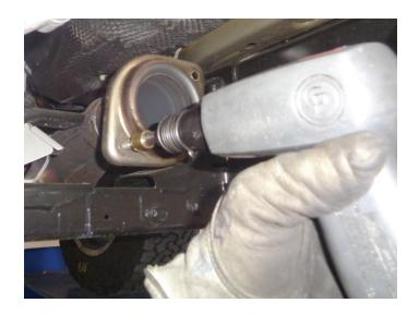
8. Remove nuts from stock and Flowmaster clamps, apply anti-seize compound to bolts and re-install nuts.
