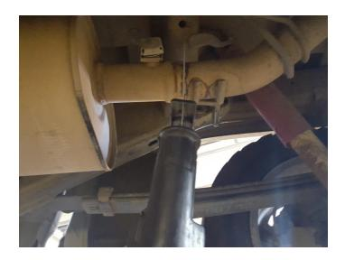
4. Dismount wire hangers (x3) from isolators and remove remaining tailpipe from vehicle.
