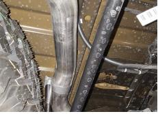
Place clamp (8) and rear hanger mount (removed step 3) onto left exit pipe (5) then connect it to y-pipe left outlet. Re-install rear hanger mount then tighten clamp just enough to allow for later adjustment.
