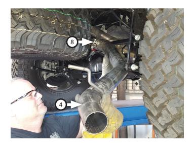
11. Insert **rear frame hanger (7)** onto right exit pipe then place it on passenger frame rail, aligned to holes. Install wiring harness bracket and bolts (x2) (from step 10) and tighten exit pipe clamp to allow for later adjustment.
