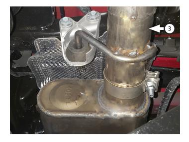
Just behind passenger rear tire, unbolt wiring harness bracket. Retain bolts (x2) for later use. Place clamp (8) onto right exit pipe (4) and connect it to y-pipe right outlet but do not tighten clamp.
