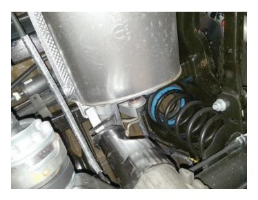
4. Loosen ball clamp, disconnect inlet pipe at catalytic converter and slide exhaust system out and down from vehicle.
