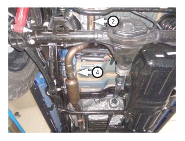
10. Place **clamp (4)** onto slip-fit of tailpipe then connect it to rear inlet pipe. Fasten mount to frame with bolts (x2) (removed step 3). Tighten clamp just enough to allow for adjustment.
