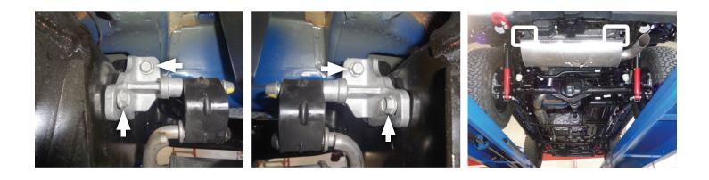
4. Loosen clamp then remove muffler from vehicle. Place it next to **tailpipe (3)** and transfer driver mount over.
