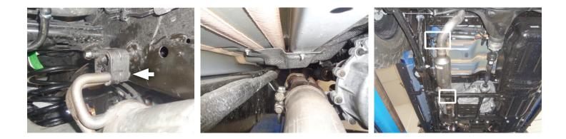
6. Rotate and remove resonator assembly from vehicle. Remove and retain its clamp for later use.
