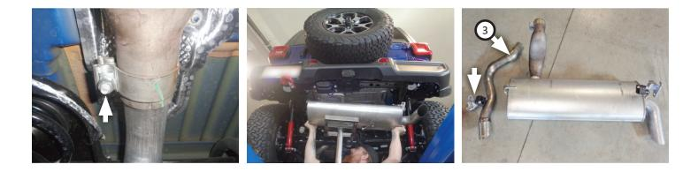
5. Remove factory rear of resonator assembly from rubber isolator then loosen bolt on clamp at inlet clamp.
