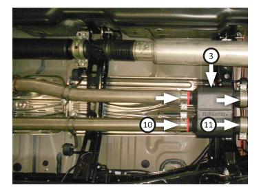
9. Connect **right and left front tailpipes (4, 5)** to muffler outlets. Tighten clamps just enough to allow for adjustment.
