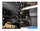
7) Slide the side exit pipes **#86097S** or the rear exit pipes **#86098S** onto the ends of both over axle pipes and place a supplied 2-1/2" clamp onto these slip-fit connections. Tighten just enough to hold in position. Place the two stainless tips **#ST461** onto the exit pipes and tighten them enough to hold position. Rotate the exit pipes and tips to the desired distance from the body or bumper, so that the angle cut on the tips are in the desired location.
