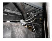
6) Place left front tailpipe section **#86094S** into position over the rear axle and slide into the left muffler outlet. Place a supplied 2-1/2" clamp onto the back of the pipe. Place left rear tailpipe section **#86096S** onto the front section, and connect the hanger welded to the rear of the pipe into the rubber hanger installed in step 3 above. Pipe should be centered between the shock and the spare tire when adjusted. Tighten the clamps just enough to hold in position.
