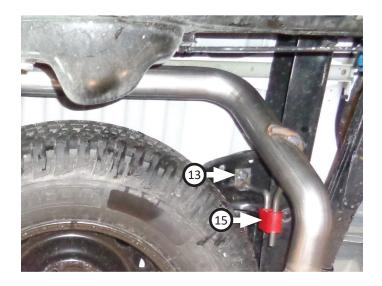
**NOTE:** This kit includes both side and rear exit pipes. A side exit is preferable for towing purposes, to avoid blowing fumes in or on vehicles you may be towing (eg: RV trailer, boat, etc). Otherwise, if you wish to equip your vehicle with a rear exit exhaust, use **rear exit pipes (7)** now in place of side exit pipes.
