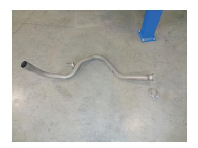
4. Remove bolts (x4) at front flange connections (x2). Disassemble wire hangers from isolators and remove muffler inlet pipe assembly. Retain bolts for later use.
